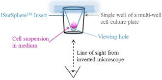
Figure 2. Schematic diagram of a single ISurSphere<sup>™</sup> insert placed in a single well of a multi-well cell culture plate depicting a drop of cell suspension in growth medium above the viewing hole.
