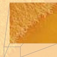
Background image: Polyesterurethane block copolymer spin coated onto a silicon wafer, low resolution, 10 \mu m. High resolution, 2 \mu m (above).
